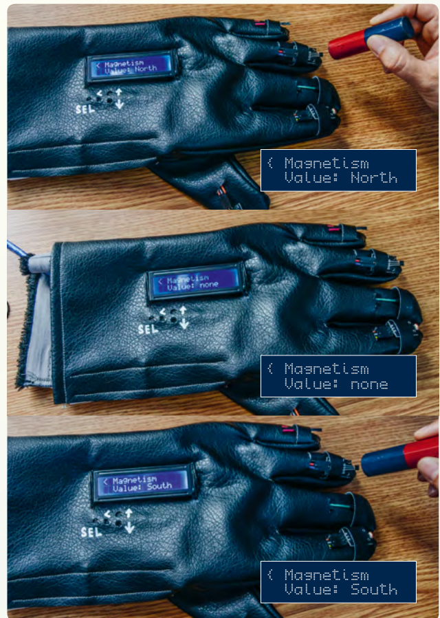
@ 1a-c: Determining the poles of a magnet
